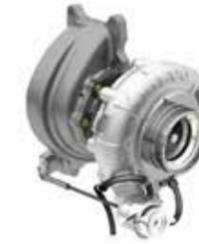
Energy is recaptured by the Turbo Compound unit from the engine's exhaust gas. The extra power captured by the TC is returned to the drive train. The Volvo integrated driveline then uses extreme downspeeding to maintain road speed at lower RPM, saving even more fuel.
