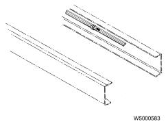
If a whole bundle of tubing needs to be repaired or lengthened, make sure the fittings are staggered instead of installed at the same length. Put the larger fittings close to a bracket for support and the smaller fittings further away.
