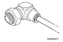
The fitting body is made of brass. An internal O-ring seals on the outside diameter of the tubing and the retaining collar holds the tubing firmly in place. Straight fittings have an internal hex grip, most others have external hex grip. A number of valves also come with push-type connectors already installed in the valve body.
