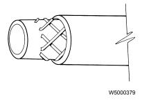
In areas where great flexibility is needed, air is routed in rubber hoses, for example, between frame and the axles. A hose is built up of three layers of rubber and reinforcement. Hoses are specifically made for each installation to the correct length with crimped on fittings on either end.
