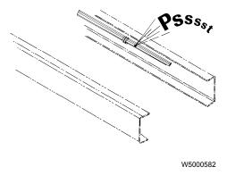
Damage to one tube is repaired so that the repair fitting is close to a bracket for support. Prepare the tubing as outlined on the previous page. Push the tubing ends into the fitting. Leak test fitting at full pressure after system pressure has been established again.
