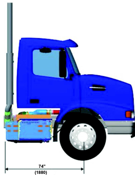
Integrated DPF/SCR with three battery box driver side and frame mounted air tanks
