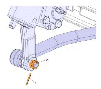
16. Position the replacement drag link rod at the steering knuckle as shown in the figure below.
