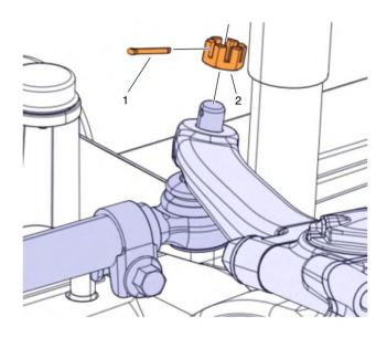
6. Using tool 9996201 (Puller), remove the existing drag link from the steering knuckle as shown in the figure below.
